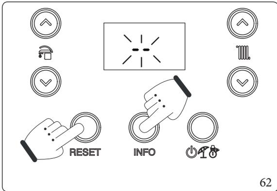
To access the programming phase, press and hold the buttons "RESET" and "INFO" for more than 5 seconds; the display shows two dashes "--" flashing and you must enter the password (69) to access the programming menus.
