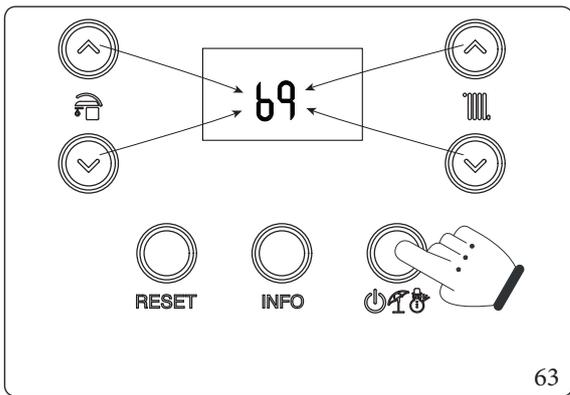
To enter the first digit use the buttons to adjust the DHW "6", to enter the second digit use the buttons to adjust the central heating temperature "9". To confirm the password and access the menu, press the operating mode button "power icon".
