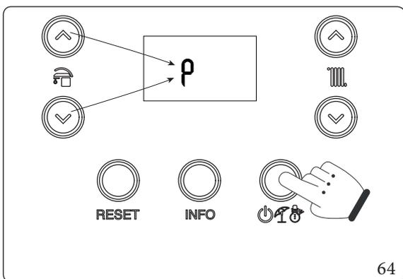
Once in the menu, you can cyclically scroll the four submenus (P, t, A, S) by pressing the DHW buttons "6", to access the menu press the button "power icon".
