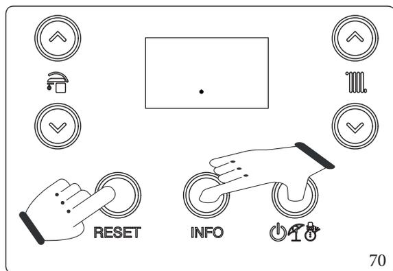
The function is activated from boiler in “off” by pressing and holding the “RESET”, “INFO” and “Power/Boiler” buttons for more than 5 seconds.
