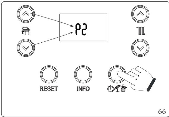
The first digit of the central indicator (Fig. 58) shows the family of the parameter, while the second digit shows its number.
