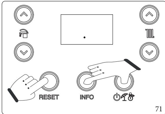
The function is activated from boiler in “off” by pressing and holding the “RESET”, “INFO” and “ON/OFF” buttons for more than 5 seconds.
