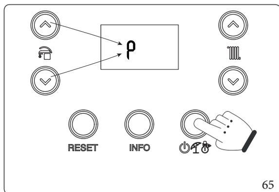
Once in the menu, you can cyclically scroll the four submenus (P, t, A, S) by pressing the DHW buttons, to access the menu press the button.
