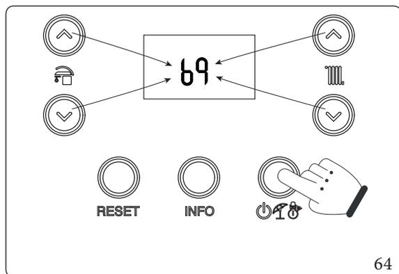
To enter the first digit use the buttons to adjust the DHW temperature, to enter the second digit use the buttons to adjust the central heating temperature. To confirm the password and access the menu, press the operating mode button.
