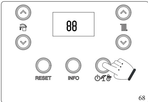
Press the mode of operation button “
