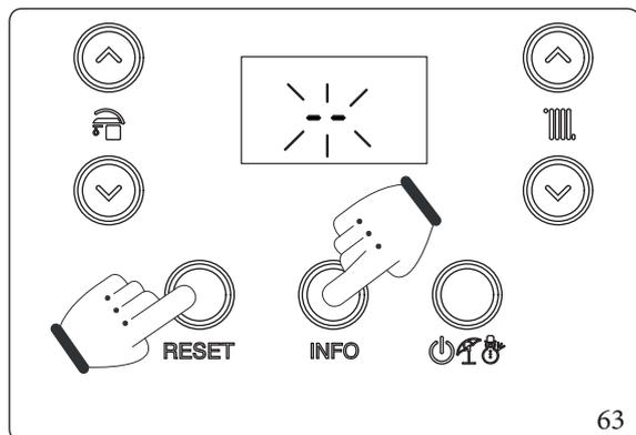
To access the programming phase, press and hold the buttons "RESET" and "INFO" for more than 5 seconds; the display shows two dashes "--" flashing and you must enter the password (69) to access the programming menus.
