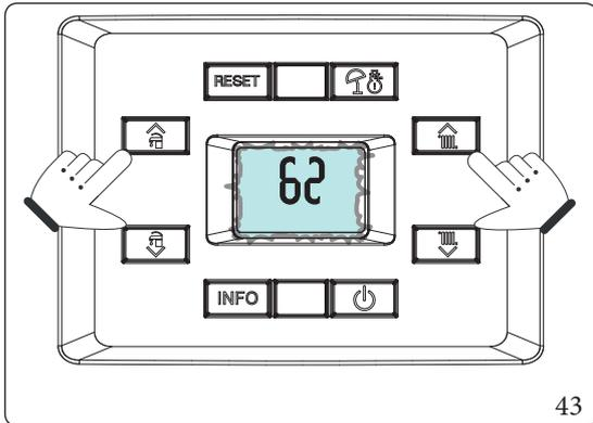
The display will show two dashes “--” flashing. Now enter the password “62” to activate the complete calibration (enter the first digit by pressing the 1-2 buttons (1-2) and the second digit by pressing the buttons 5-6 (5-6)).
