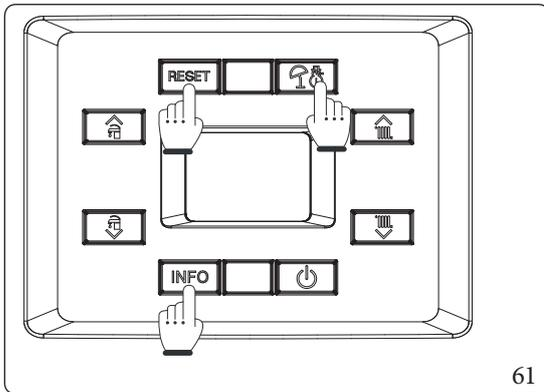
The function is activated from boiler in “off” by pressing and holding the “RESET”, “INFO” and “
