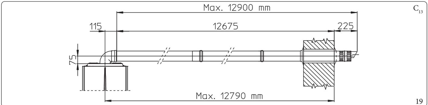
**Mounting the horizontal intake-exhaust kit Ø 80/125 (Fig. 20)**
