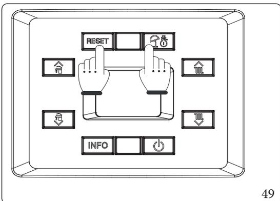
Press and hold buttons “RESET” and “10” for more than 5 seconds.
