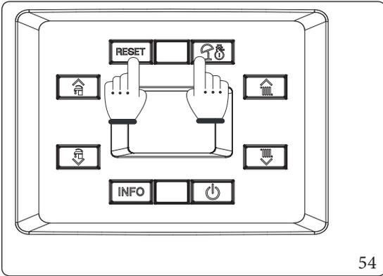
To access the programming phase, press and hold the buttons “RESET” and “
