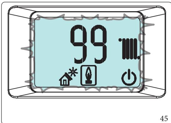
Only after the “Flame” symbol flashes is it possible to change the CO<sub>2</sub> value (Par. 3.10) or switch to the next heat output parameter by pressing the “Power” button.
