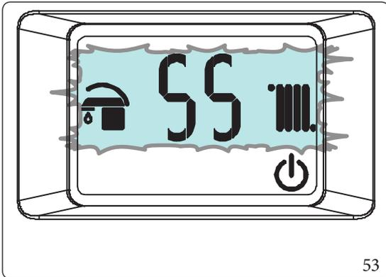
To activate the function, press the buttons "RESET" and "⏻" simultaneously until function activation, which is displayed by indicating the fan operation speed (in hundreds of revs) and ignition of the flashing "🔥" and "🌀" symbols.
