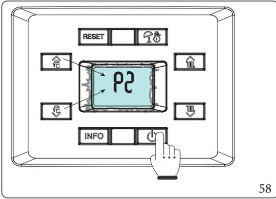
The first digit of the central indicator (  $\text{P}$  ) shows the family of the parameter. The second digit shows the parameter number. Press the “  $\text{P}$  ” button to display the value of the selected parameter.
