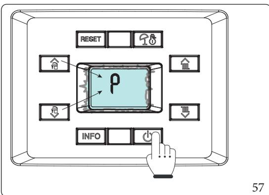
Once in the menu, you can cyclically scroll the submenus by pressing the D.H.W. buttons “
