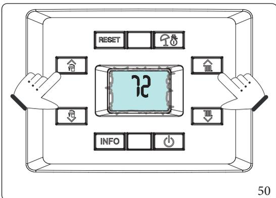
The display will show two dashes “--” flashing. Now enter the password “72” to activate fast calibration.
