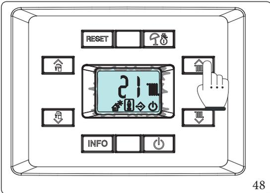
To increase the combustion setting, press the button 5 () , to decrease it, press the button 6 (). As the combustion setting increases, the CO<sub>2</sub> value decreases and vice-versa.
