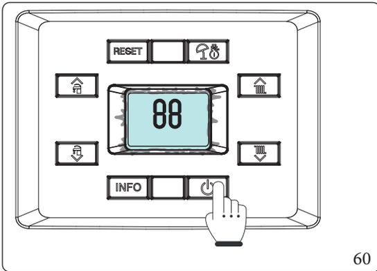
Press the mode of operation button “  $\text{P}$  ” for more than 1 second to store the parameter value; confirmation is given by the word “  $\text{88}$  ” which appears for 2 seconds. If you want to exit a parameter without changing its value, press the button “ **INFO** ”. Exit the programming mode by waiting 15 minutes or by pressing the “ **INFO** ” button until you return to the desired display.
