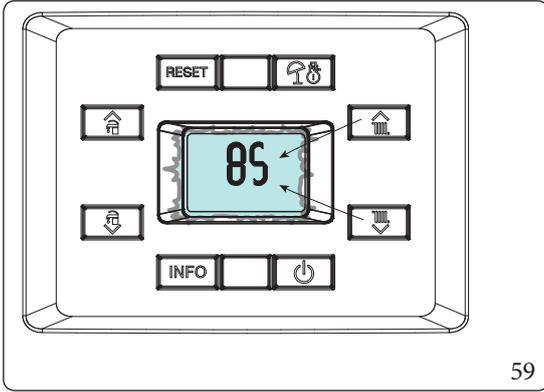
Its value can be adjusted by using the central heating temperature adjustment buttons “  $\uparrow \downarrow$  ”.
