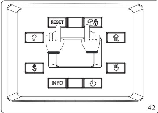
Press and hold buttons “RESET” and “1-2” for more than 5 seconds.
